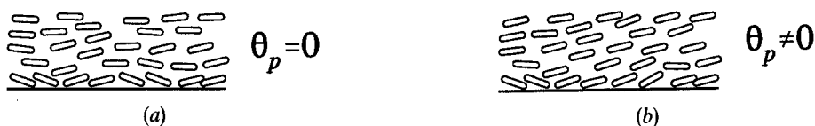
Figure 3. Illustrative drawing of the bulk pretilt \Theta_p formation in the case of zero orientation ( a_1 = 0 ) (a) and non-zero orientation ( a_1 \neq 0 ) (b) of the azimuthal distribution function of the monolayer.
